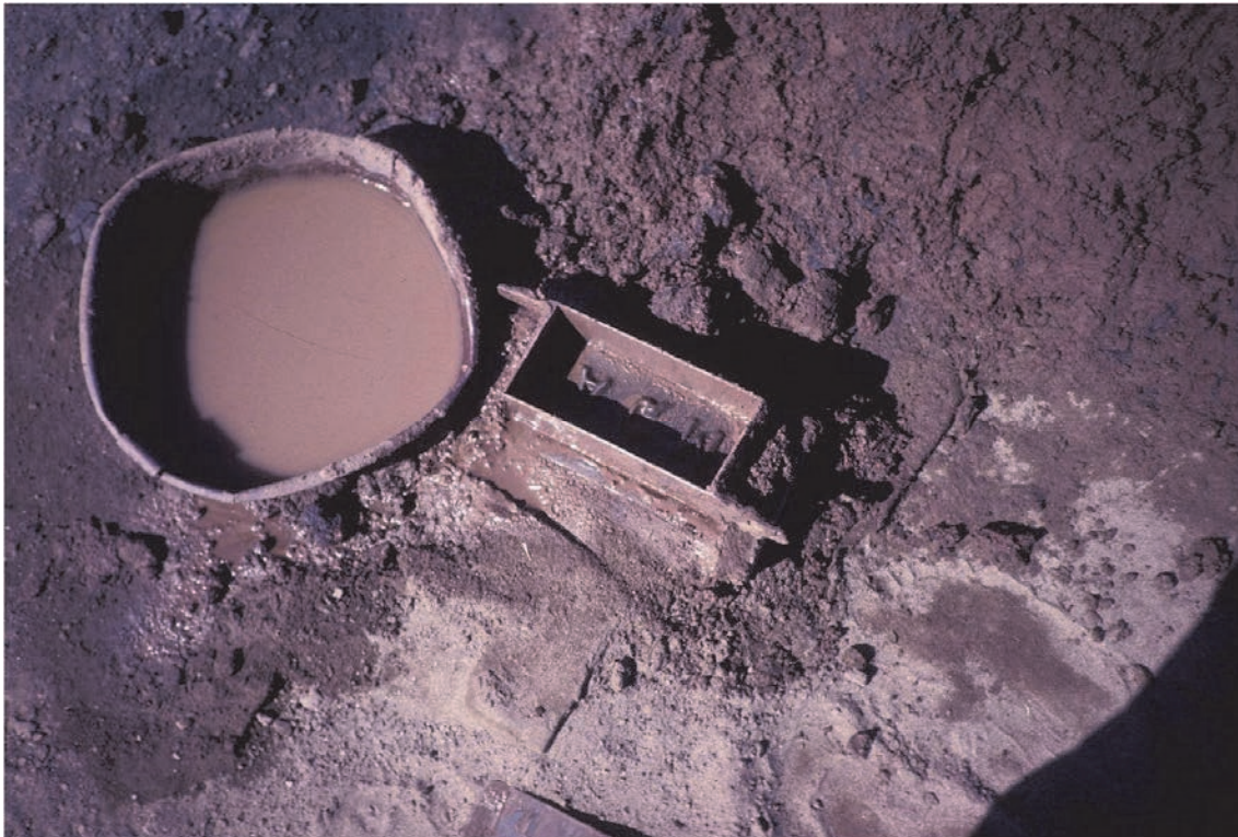
Figure12: Brick mould for modern brick production in Gilund (Courtesy: Shinde et al. 2014)
